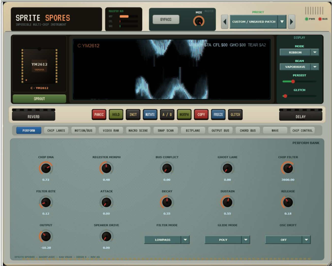
FIG 3 The Perform bank: four character knobs on the top row, filter and envelope below, voicing and output at the bottom.
