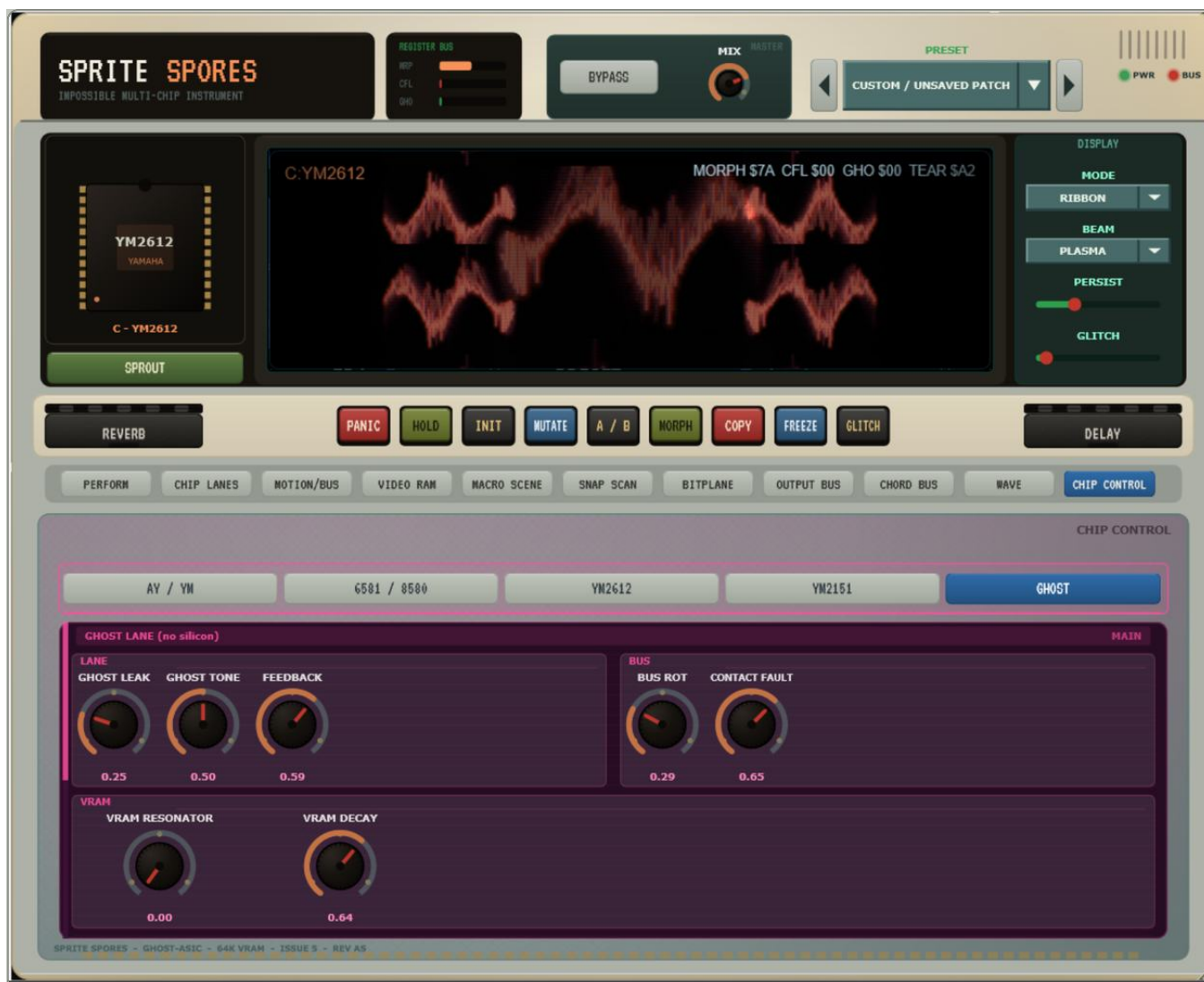
FIG 10 The Ghost page – lane, bus and VRAM sections. No engine control, because there is no chip to model.
