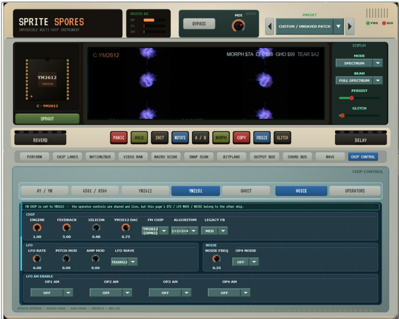
FIG 8 The YM2151 page with FM Chip set to YM2612 – the cyan banner across the top says so, and names which controls belong to the other chip.
