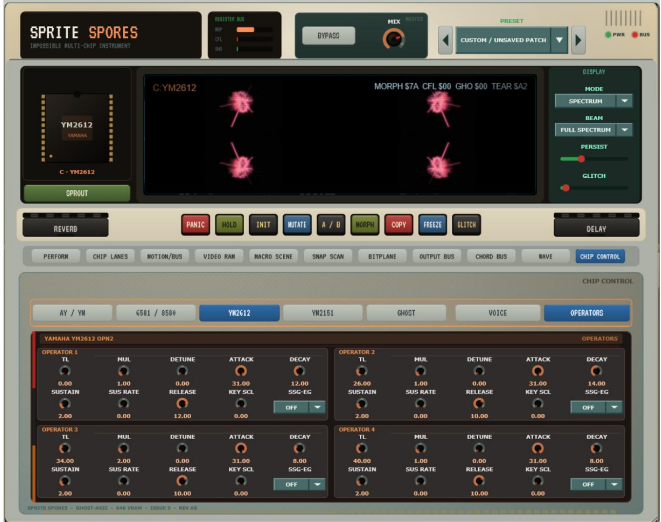
FIG 7 The Y2612 Operators tab. Four operators, identical layout, SSG-EG on each. (Captured before the dB readout; TL now reads in decibels below full scale.)
