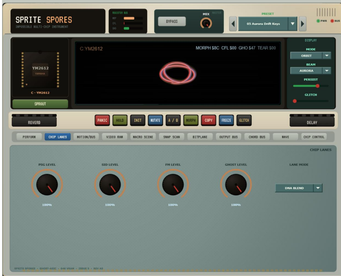
FIG 2 The Chip Lanes page. Four lane faders and the Lane Mode selector, here set to DNA Blend.
