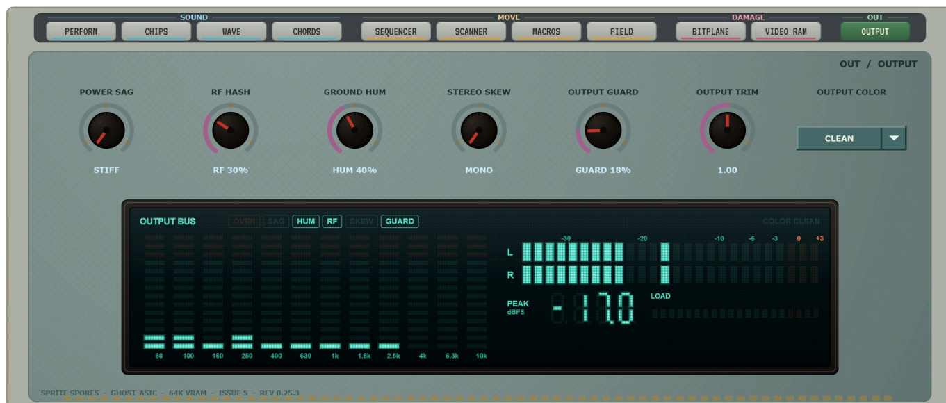
FIG 20 The OUTPUT BUS monitor: 12-band spectrum, L/R meters with peak hold, a PEAK readout in dBFS, LOAD, and lamps for OVER and each active stage.
