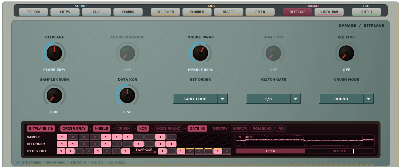
FIG 19 The chain lights the stages in use and shows a sample word with its dropped bits struck out.
