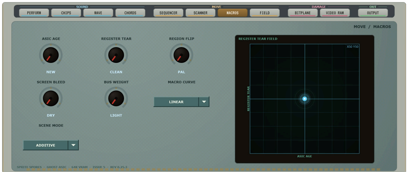
FIG 18 The REGISTER TEAR FIELD pad moves ASIC AGE (across) and REGISTER TEAR (up) together and leaves a trail.
