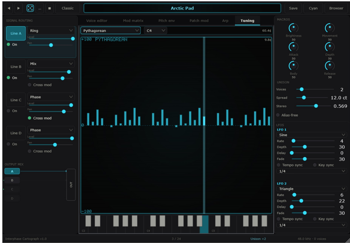
The Tuning tab set to the Pythagorean temperament, rooted on C4. Each bar shows that note's offset from standard 12-TET pitch.
